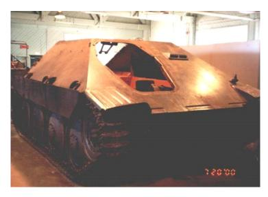
A frontal view of the Hetzer. As you can see, the entire main armament and mantlet have been removed for separate restoration. The tank has been sandblasted right down to the original grey primer. The interior has also been blasted down to the red oxide primer that was applied over the bare steel before the characteristic German Elfenbein ivory white colour was applied. Seen through the opening for the main gun is the travel lock that was fastened to the ceiling of the fighting compartment.
