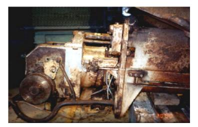
The main gun. A great detail view of the 75mm PAK 39 main armament. All of the original stenciling can still be seen clearly on the gun and all over the vehicle. This has been meticulously recorded by the restoration team and will be re-applied after the interior is complete. All operating mechanisms for the gun are still there and still work properly too. The breech block retains its coat-
